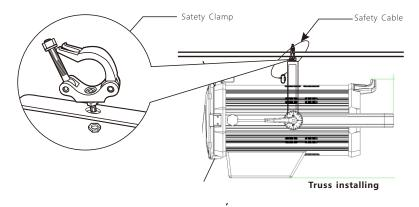
Regardless of the rigging option you choose for your PROFILE NF 200CW, always be sure to secure your fixture with a safety cable. The fixture provides a built-in rigging point for a safety cable on the hanging bracket as illustrated above. Be sure to only use the designated rigging point for the safety cable and never secure a safety cable to a carrying handle.
